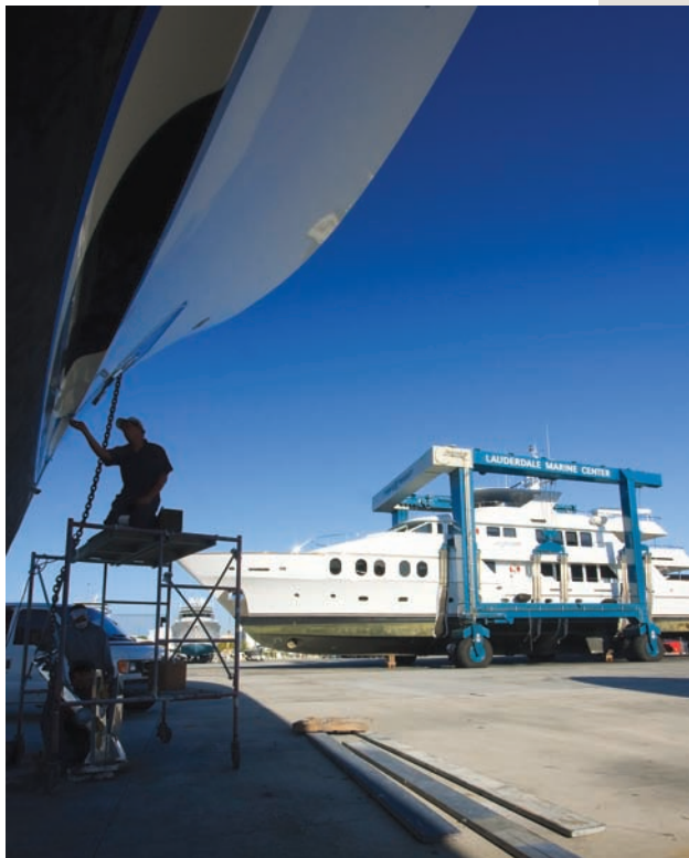
Lauderdale Marine Center travel lifts can handle up to 330 tons for haul out and launches.
